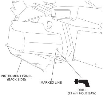
Position the remote control sub harness as shown 8. and mark this position.
