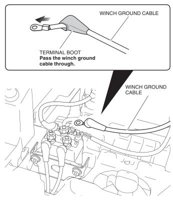
44. Install the winch ground cable as shown.
