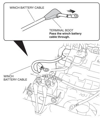
42. Install the winch battery cable as shown.
