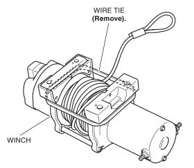
28. Install the winch to the winch bracket as shown.
