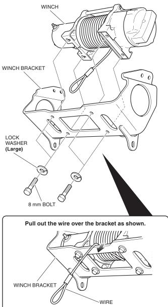
29. Loosely install the assembled winch as shown. <**Front side**>
