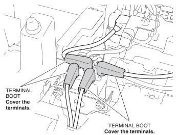
46. Install the contactor cover as shown.
