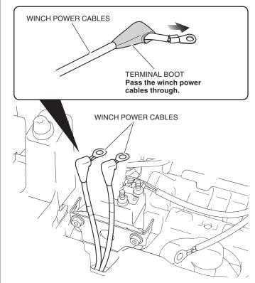
36. Install the winch power cables to the corresponding color terminal on the contactor as shown.
