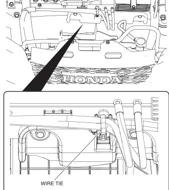
23. Reinstall the coolant reserve tank in the reverse order of removal.
