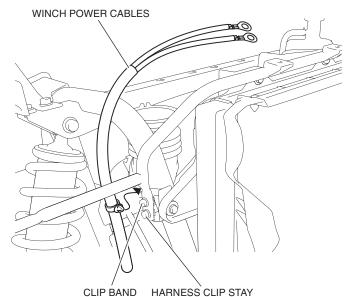
20. Secure the winch power cables with the wire tie as shown.
