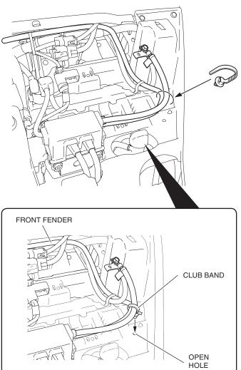
48. Secure the winch ground cable and sub harness with the wire tie as shown.
