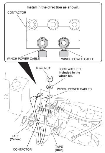
NUT VEHICLE'S HARNESS STARTER RELAY
