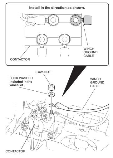
45. Cover each cable terminal with the terminal boot as shown.
