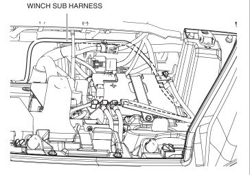
34. Connect the sub harness to the contactor as shown.
