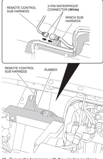
18. Secure the harnesses with the wire ties as shown.
