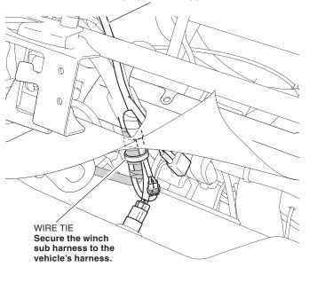
17. Connect the winch sub harness and remote control sub harness as shown.
