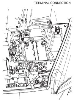
32. Route the winch power cables through the hole in the front fender as shown.
