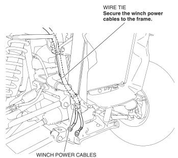
25. Install the winch power cables as shown.
